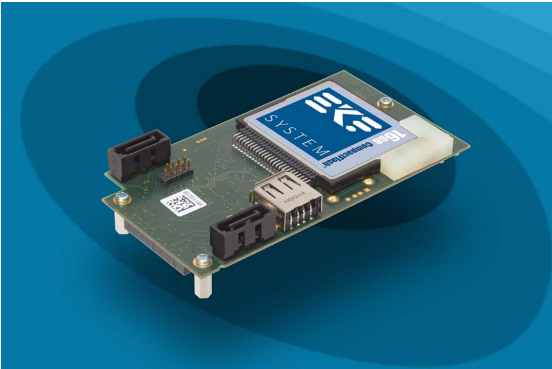
C40-SCFA • CompactFlash® Card Holder
